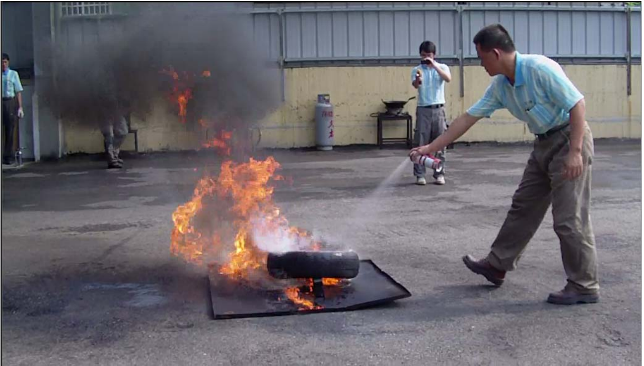
3. Extinguishing by one can of Fire Buster X400; Highly toxic black smoke (Dioxins)
